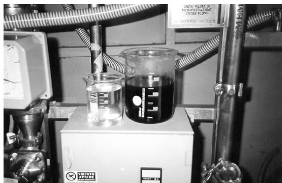
Fig. 3. Photograph of samples before (right cylinder-feed) and after nanofiltration process (left cylinder-permeate).
